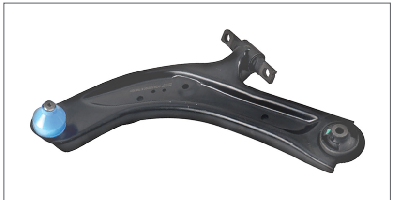
The SKF blue cap identifies the new synthetic grease in the track control arm
